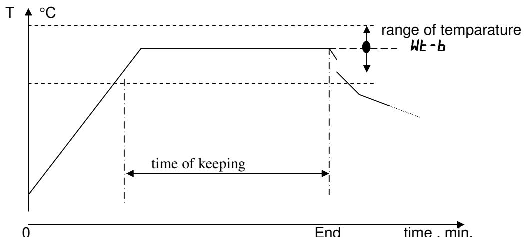
**AT**: automatic selection of parameters (parameters of PID combination:  $P$ ,  $I$ ,  $d$ ) of temperature regulation (further in text: AT). If the temperature in the chamber of furnace changes and is unstable it is required to switch on AT. AT can be switched on only when regulator executes the program.
